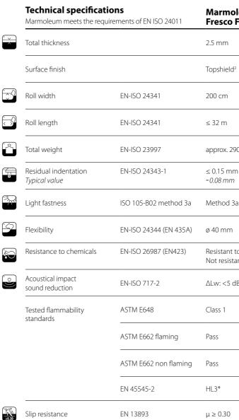
\*EN45545-2 testing has been carried out on different substrates/adhesives. This is the highest achieving result. For a full overview of specific results on aluminium and plywood subfloors please ask.
